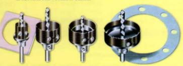
Required hole size should be drilled by mounting appropriate Hole Saw Cutter on Electric Power Drill or Bench Drill. Place softwood bebeath Hole Saw Cutter to avoid damage.
