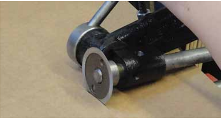
(Figure 6) To cut the OD, engage the top cutting disc by rotating the cutting disc lever clockwise. The top cutting disc should now penetrate the gasket material and is now in the proper position for cutting.
